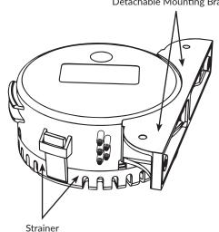
\*The BG-One can also be mounted on the hull using three #8x0.75" 316 stainless steel screws. Mount the strainer first, then attach the BG-One into place.
